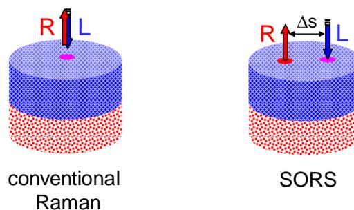
Figure 1: Schematics of conventional Raman and SORS sampling configurations.
